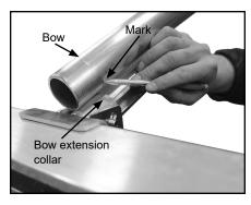
IMPORTANT: Make cut perpendicular to bow. Do not cut end of bow with factory drilled hole.
