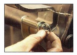
Rotate tarp stop to locked position, insert pin and clevis as shown on front tarp stop.
