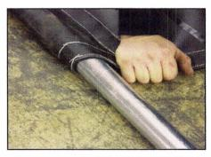
Insert the 2" roll pipe open end first into pocket from rear of tarp and slide through to other end. Leave 18" (length varies) of gudgeoned end out at rear of tarp.
