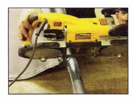
Install "U" clamps on overlapping heat seal seams. Cut off excess roll pipe flush with pocket at front end of tarp.
