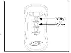
**Momentary mode (switch setting 7):** Press and hold Open to roll tarp fully open. Press and hold Close to roll tarp closed.
